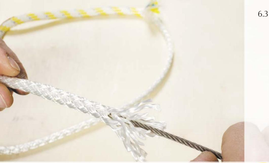
Insert the wire into the core to a distance of approx. 70 cm.
