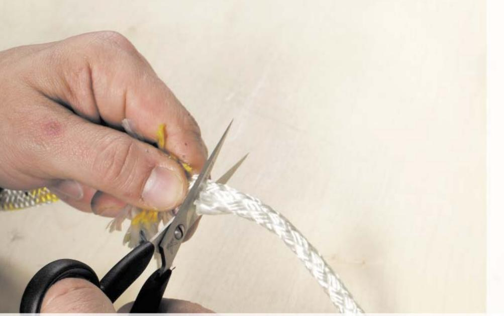
Pull approximately 20 cm of core out of the cover and cut off. Then holding onto the end of the core slide the cover back approx. 3 m.
