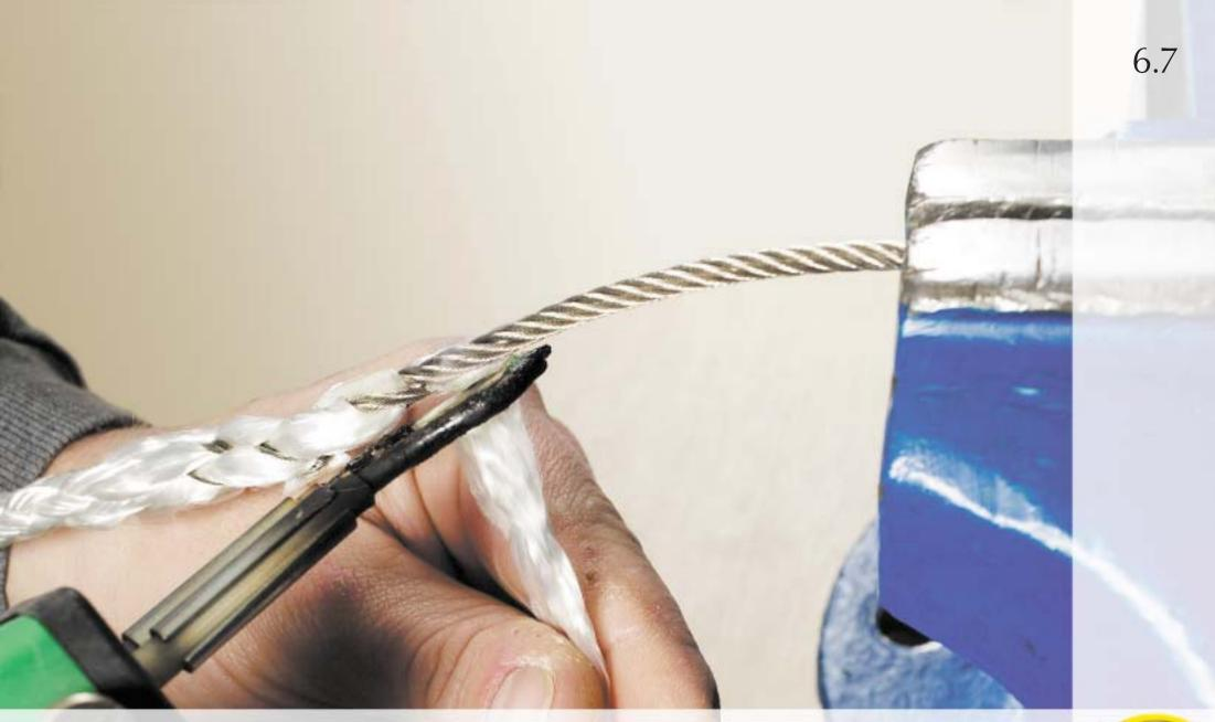
Trim away the ends of the rope using a hot knife.
