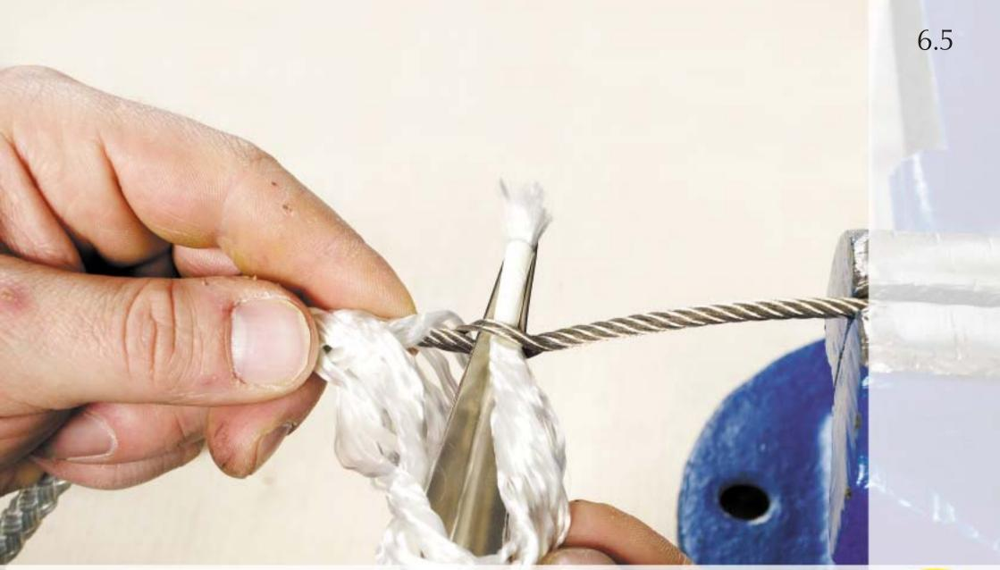
Using the fid pull the first strand through under two strands of wire.
