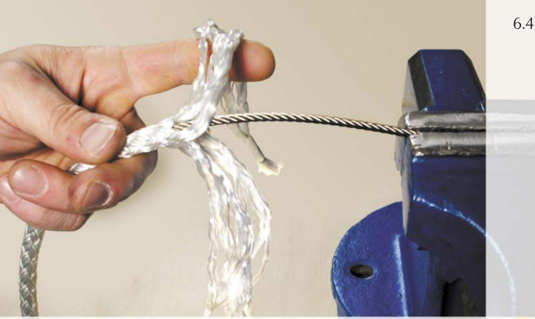
Hold the wire in a vice and unravel the core for 15cm. Than make the strands into roughly 3 equal strands.
