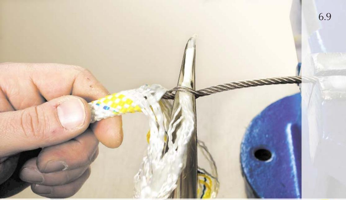
Now splice the cover into the wire in the same way as the core was spliced into the wire.
